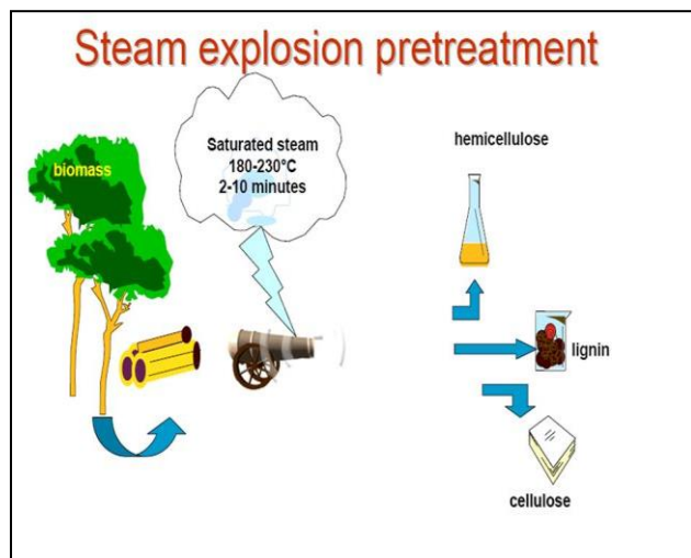
Fig. 4 (a) Steam explosion pretreatment cellulosic biomass via steam explosion.
